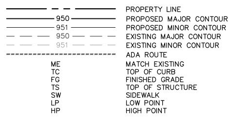
950 PROPOSED MAJOR CONTOUR MATCH EXISTING TOP OF CURB FINISHED GRADE TOP OF STRUCTURE SIDEWALK LOW POINT HIGH POINT
